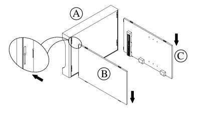
Step 2. Carefully align male and female bracket to connect left side panel B, right side panel C with back frame E, push the back frame E down to lock these panels in place.
