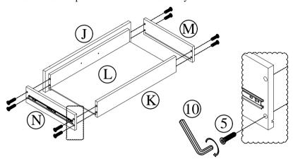
Step 12. Pull out the ball bearing slides and carefully align the slides on drawer box with slides pre-installed on side panel/partition panel then insert drawers. If the drawer fronts mis-align please loose the screw that holding drawers slides on outside of the drawer box and make proper adjustment then fasten these released screws.
