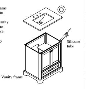
Step 14. Place the vanity in the desired location. Ensure the vanity set leveled by slightly adjust the adjustable levelers. Install the faucet and all plumbing. Ensure there are no water leaks.
