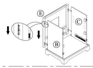
Step 3. Carefully align male and female bracket to connect left side panel B, right side panel C with front frame D, push the front frame D down to lock these panels in place.
