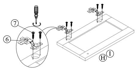
Step 7. Carefully hold the door H/I and make sure screw holes on door hinge base align with predrilled screw hole on inside of side panels, use philips head screw driver and screw #7 to attach door hinge #6 on inside of side panels. Adjust the screw on center portion of hinge slightly by loose or fasten screws to make sure even gap around door, and close the 2 covers on the door hinge #6.
